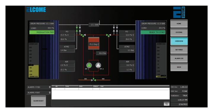
Elcome, in collaboration with Gronne Technologies, has developed a distributed control system (DCS) based boiler automation system to take full advantages of a plant's productivity and improve operations by precisely controlling fuel and combustion air. The result is maximum efficiency gain, reduced operating costs and lower emissions to the atmosphere.
